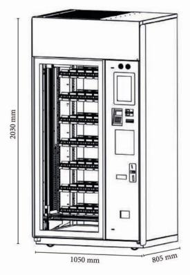
Width 1050 mm Depth 805 mm Height 2030 mm Weight (with 6 floors) 250 Kg Maximum number of floors Selections maximum per floor Type of lighting high-brightness LEDs (25 W) Power supply 100-240 V | 50/60 Hz Indoor temperature -25 °C **Energy consumption** 600 W (with the lowest temperature)
